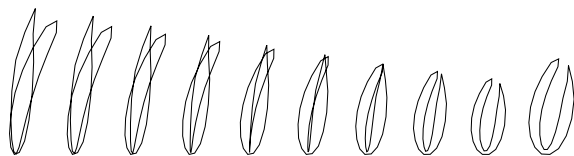
Figure 5: Evolution from a random initial shape with self-intersections (left) to an aligned final shape (right) during gradient ascent.
